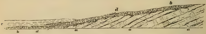
FIG. 212.—SECTION OF PART OF THE FLANK OF THE MENDIP HILLS ( B. ), showing the Carboniferous Limestone ( a a ) overlaid by dolomitic conglomerate ( b b ) and that by red marls ( c ).
